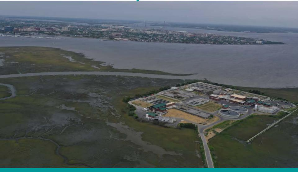
36 MGD Conventional Activated Sludge Treatment Plant
