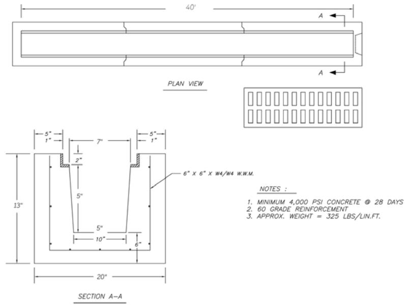
**Figure 18:** Trench Drain Schematic (Adapted from Precast Concrete Sales)
