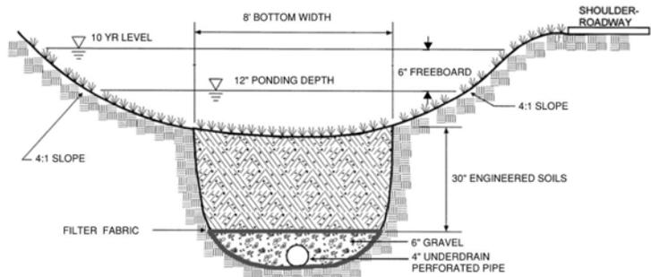
Figure 16: Width Cross-section of a Dry Enhanced Swale (Gwinnett, 2020, Vol 2 pg 222)
