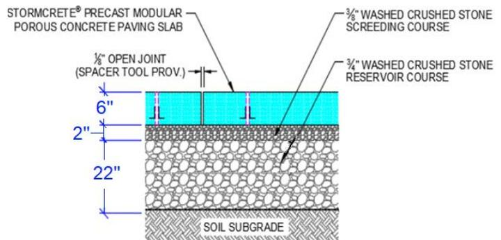
Figure 12: Stormcrete schematic (Stormcrete, 2021)
