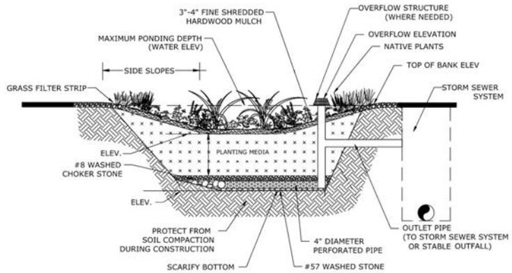
Figure 9: Bioretention Schematic with Underdrain (Gwinnett, 2020, Vol 2 p.166)
