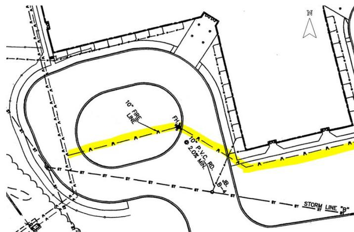
Figure 7: As-Built Drawing for Bus Loop with Fireline Highlighted (Eberly, 2002)
