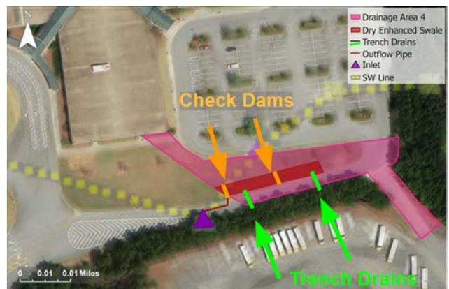
Figure 15: Alternative 4 Drainage Area for Swale (Esri, n.d.; Gwinnett County GIS, 2020)
