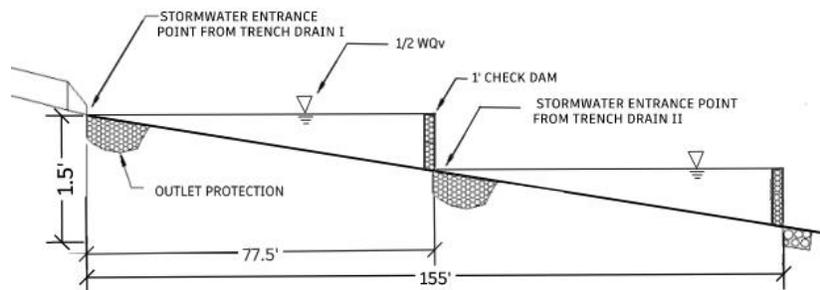
Figure 17: Length Cross-section of a Dry Enhanced Swale (Adapted from the Minnesota Stormwater Manual)
