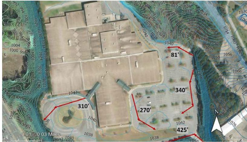
**Figure 4:** Flow Path Lengths per Basin (Esri, n.d.)
