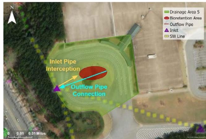
Figure 6: Drainage Basin treated by Alternative 1 (Esri, n.d; Gwinnett County GIS, 2020)
